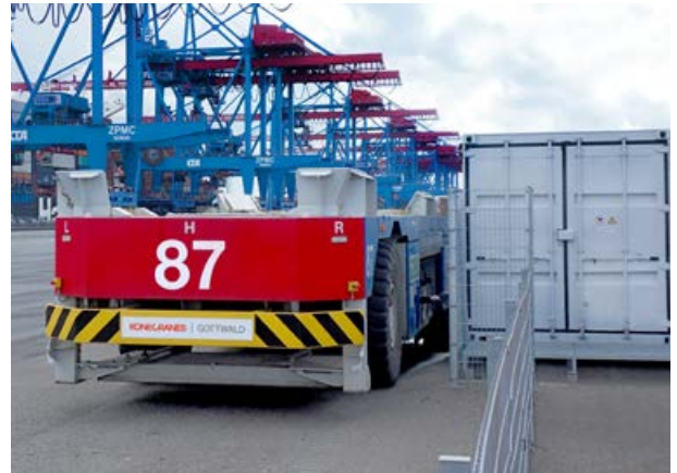
Konecranes Gottwald Li-ion Battery AGV being re-charged with an automated quick charger
