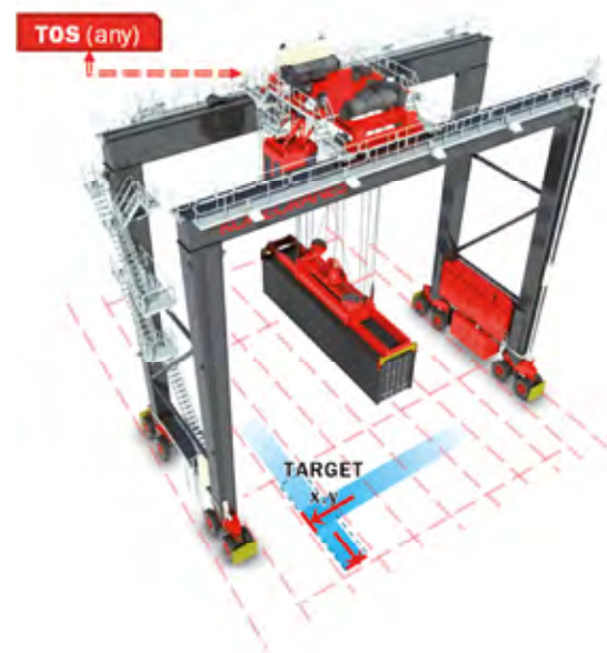
Figure 14. Auto-Positioning helps make load movements more precise.
