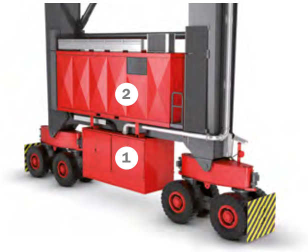
Figure 2. The diesel fuel saver is retrofitted in the genset enclosure (1) while the necessary modifications to the electrical systems are made in the e-house (2) above it. Some software modifications are also done at the same time.
