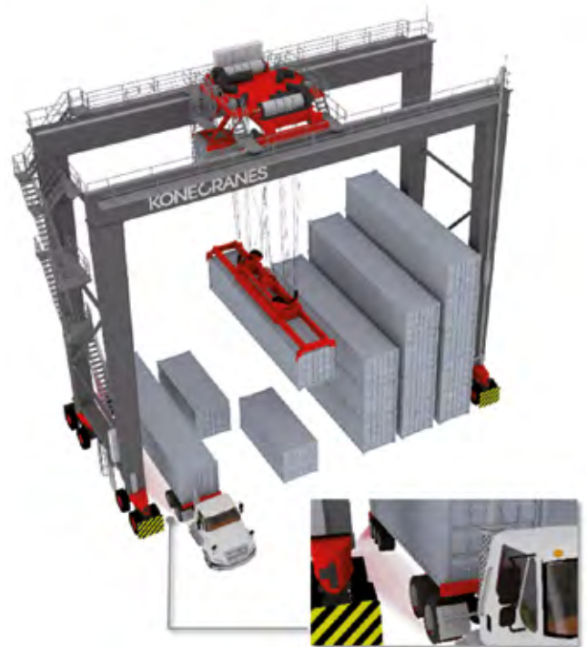
Figure 11. All twist locks must be disengaged before lifting. Trailer Lift Prevention stops lifting if a trailer lift by monitoring the trailer wheels.
