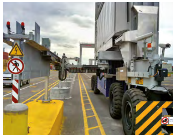
Figure 5. The Georgia Ports Authority (GPA) operates over 120 Konecranes RTGs including the fully electric busbar RTG pictured here at the Port of Savannah. The GPA plans to operate over 150 fully electric RTGs by 2022 via purchases of new electric RTGs and retrofitting existing RTGs.
